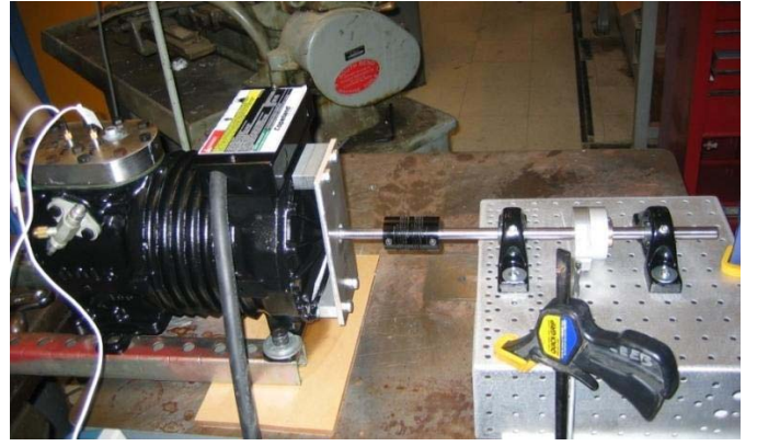
Fig. 4. Compressor test rig with shaft encoder installed on rotor extension.
