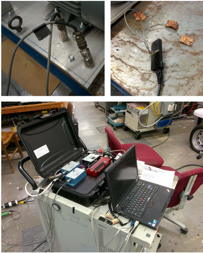
Fig. 13. Entire equipment set of [27] that VAMPIRE makes obsolete and replaces: commercial accelerometers (top left); standalone back-EMF sensors (top right); data acquisition blocks, data storage, data network, data wiring, power supply, and power wiring (bottom).
