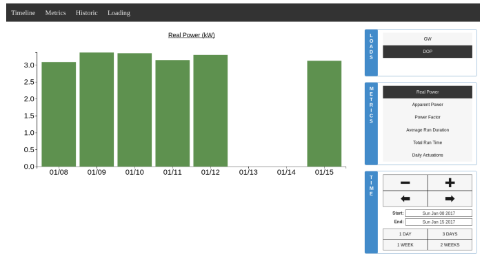
Fig. 6. The Historic View shows the daily trend for a given metric over a period of time.
