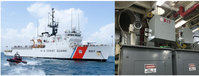
Fig. 1. U.S. Coast Guard cutter ESCANABA [13] and nonintrusive load monitoring installation onboard the ship.
