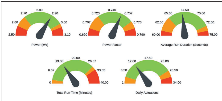
Fig. 2. NILM dashboard Metrics view indicating healthy graywater pump operation.
