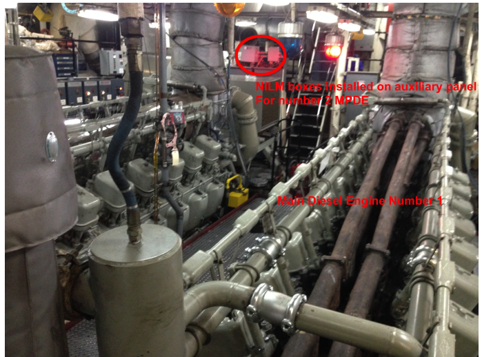
Figure 4. USCGC SPENCER engine room. Nonintrusive monitors are installed forward of the #2 MPDE just above the monitored panel.
