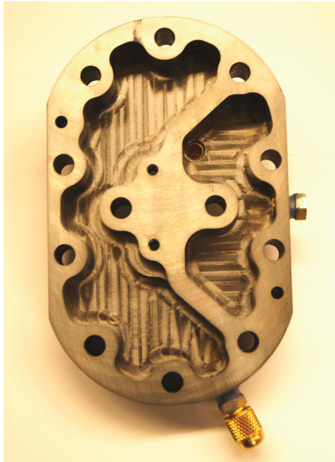
Figure 5: Picture of modified head for pressure instrumentation and slugging apparatus.
