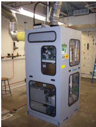
Fig. 2: A 5 kW Siemens / Fuel Cell Technology stack used for testing.
