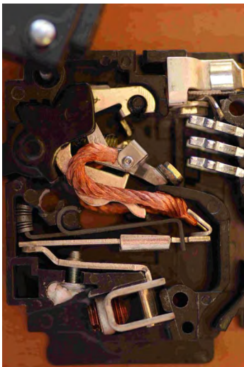
Fig. 2: A cross-section of a typical circuit breaker.
