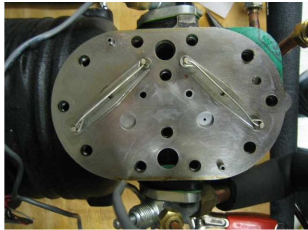
Figure 6b: Suction reeds installed in compressor with valve plate.
