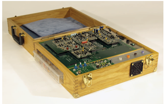
Fig. 2. An overall view of the power electronic controller kit. The wooden box houses the motherboard, on which the various controller circuit blocks are mounted. The box also has a place for storing the kit components.
