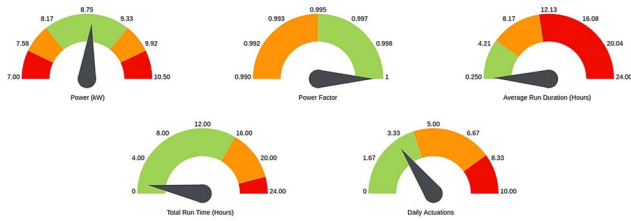
Fig. 12. NILM dashboard showing a healthy MPDE jacket water heater condition. All gauges are within the green regions.
