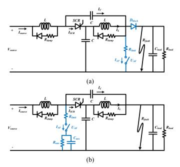
Figure 7. Two ways of manually tripping the Z-source breaker. (a) inducing an external artificial fault near the output and (b) inducing an internal artificial fault within the Z-source breaker.
