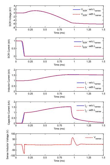
Figure 10. Fault clearing waveforms demonstrating negligible effects from the current sense inductor on the normal operation of the Z-source breaker.
