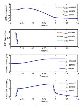
Figure 3. Fault clearing waveforms for the three Z-source circuit breakers. Waveforms for the parallel-connected and series-connected are shifted right by 10µs and 20µs respectively for clarity.
