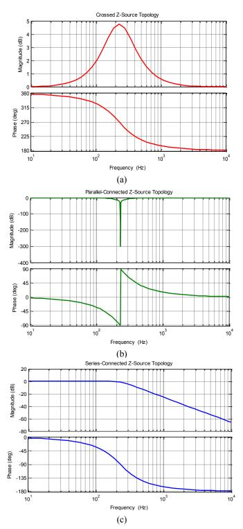
Figure 6. Input-output voltage transfer function of the Z-source circuit breaker assuming resistive load. Component values are  $R = 6\Omega C = 200\mu$ F, and L = 2.4mH.
