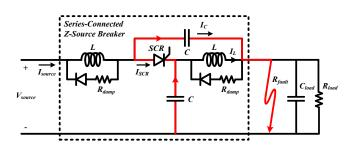
Figure 2. New series-connected Z-source circuit breaker topology.
