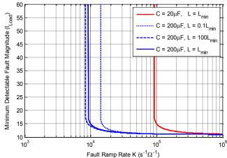
Figure 5. Minimum detectable fault magnitude vs fault ramp rate with fixed load to Z-source capacitor ratio of 5 and a load resistance of  $6\Omega$ .
