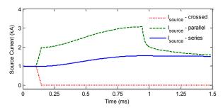
Figure 4. Comparison of the reflected fault current at the source among the three Z-source circuit breaker topologies.
