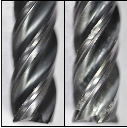
Fig. 12. Good and bad 8-mm carbide end mills.
