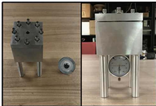
Fig. 10. Fixture for diaphragm damaging.
