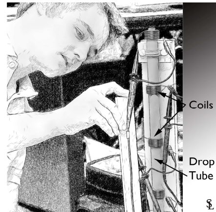
Fig. 2: Student completing preparatory measurements before dropping magnet through coils.
