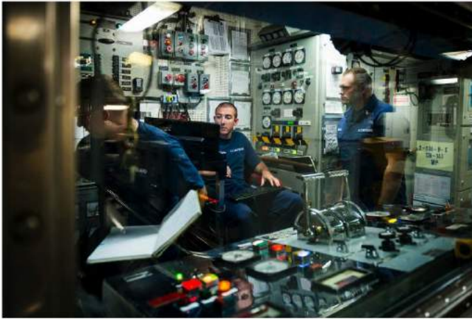
Figure 1. Typical USCG engine room watch. Notice the logbook, termed the "rough log," used to keep machinery operation times and log critical events. Also note the watchstanders monitoring equipment while simultaneously attempting to maintain logs.
