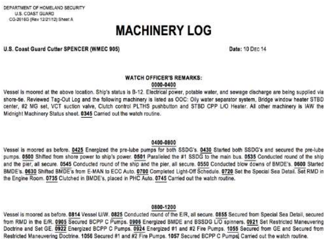
Figure 17. The machinery log generated manually by the ship's crew by logging events and times.
