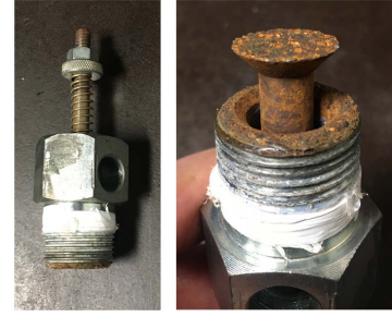
Fig. 24. Deteriorated vacuum relief valve.
