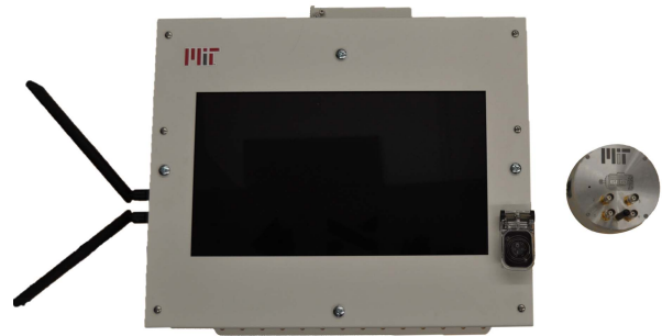
Fig. 5. Wi-Fi-enabled NILM alongside the wireless sensor platform.
