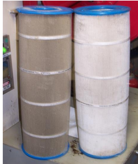
FIGURE 11. Filters used in the field experiments conducted aboard the Escanaba . The filter on the left shows considerable contamination and wear.
