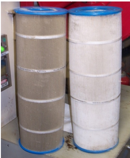
FIGURE 11. Filters used in the field experiments conducted aboard the Escanaba . The filter on the left shows considerable contamination and wear.
