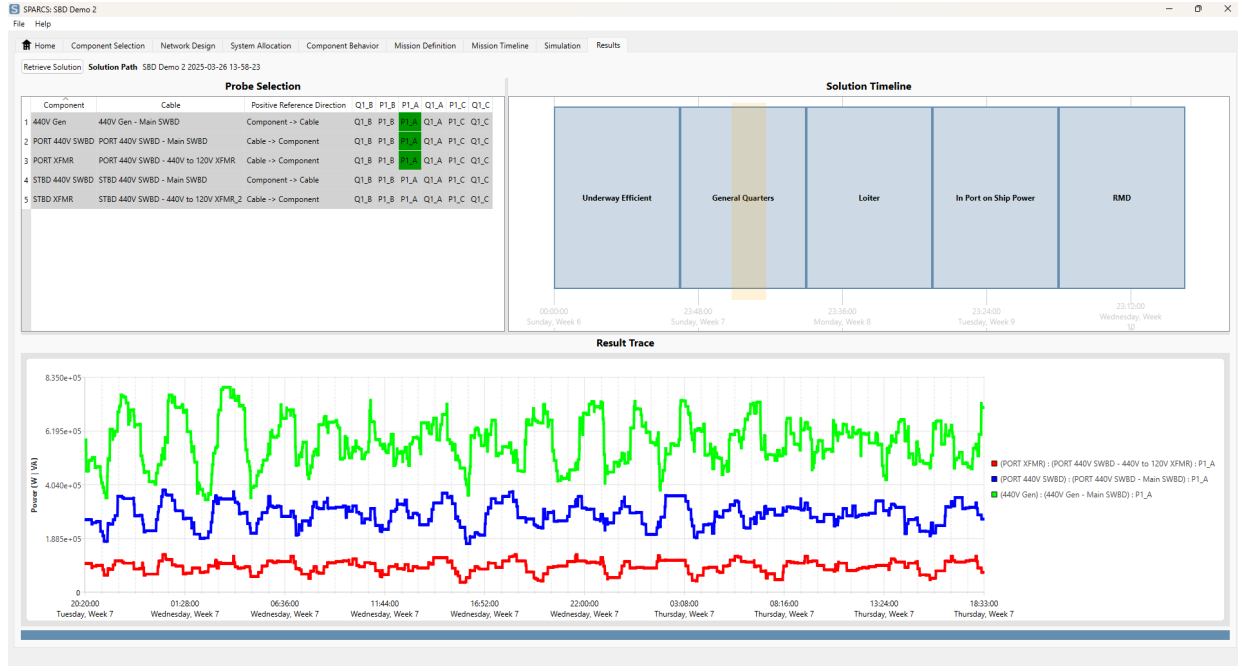
Fig. 7: Sample results during the General Quarters mission. The phase A real power trace is shown at the port transformer (red), port 440 Volt switchboard (blue), and the generation probe points (green).
