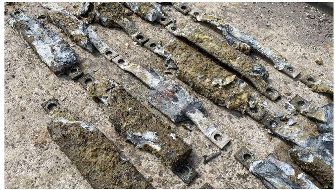
Fig. 15. Heavily depleted area zinc anode after one year.
