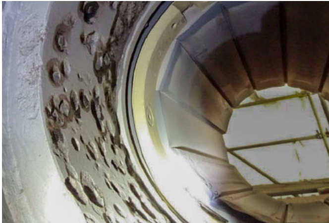
Fig. 2. Severe ship stern tube corrosion in the form of pitting.
