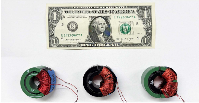
Fig. 8. Uninstalled harvester assemblies with US 1 Dollar bill for size reference. (Left to right: Nanocrystalline, Silicon-Steel, Hybrid.)
